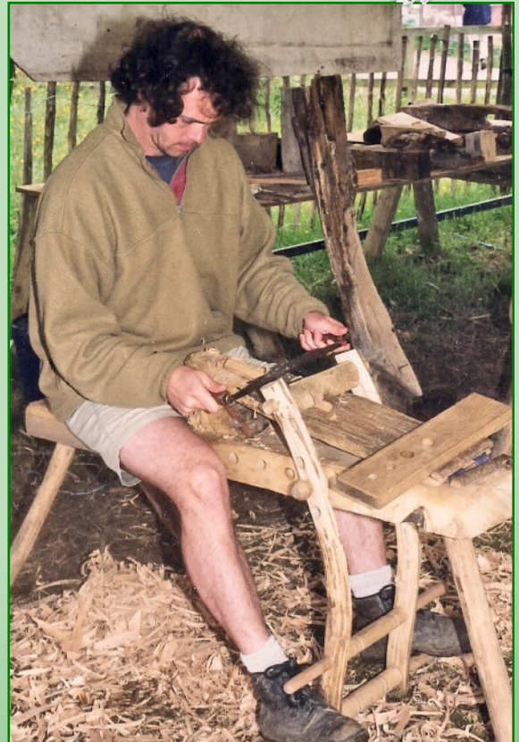
Bench for clamping and shaving pegs using a draw knife.
